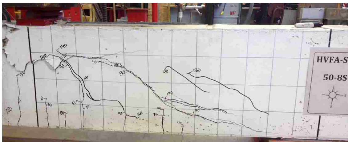
Figure B-7. Ultimate Shear in Specimen 50-8S
