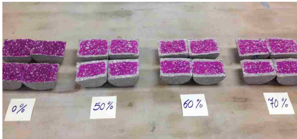
c) Specimens after Spraying the phenolphthalein pH indicator
