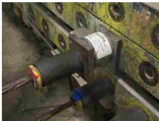
Figure F-2. Load Cell Installation Detail
