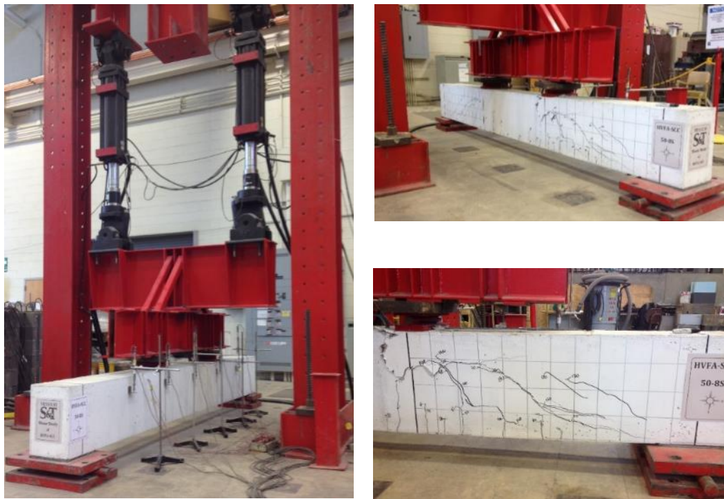
Figure 3. Test setup, instrumentation, and testing and failure mode of a beam specimen
