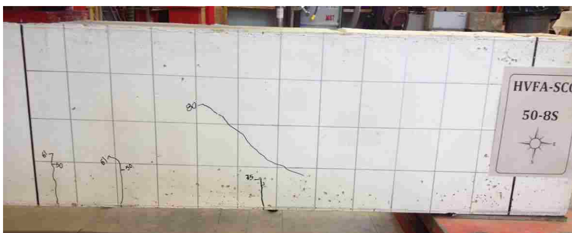
Figure B-6. Cracking Shear in Specimen 50-8S
