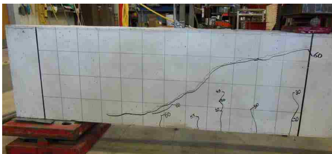
Figure B-18. Cracking Shear in Specimen 70-6N
