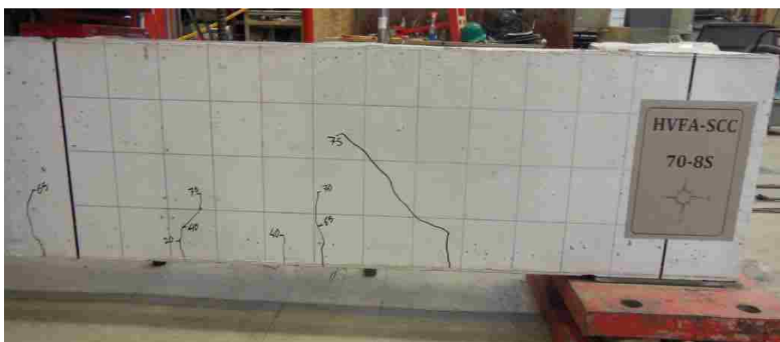
Figure B-22. Cracking Shear in Specimen 70-8S
