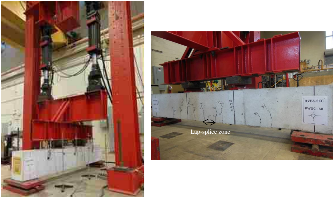
Figure 2. Test setup, instrumentation, and testing and failure mode of a beam specimen.
